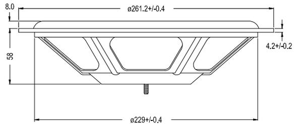
SP25R is a 25cm (10") passive radiator intended for use, as an alternative to the vented port in a bass reflex cabinet, together with an active woofer of similar size or smaller.
