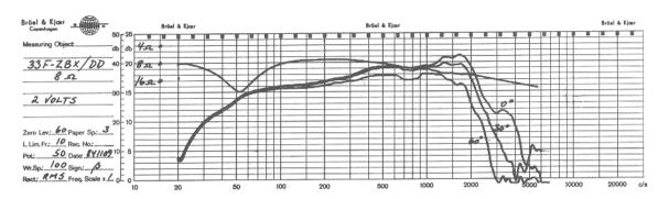
B Sound pressure and distortion on axis. The distortion components are raised by 20 dB:
