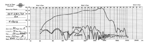
C Sound pressure response to 4 Volts step function:
